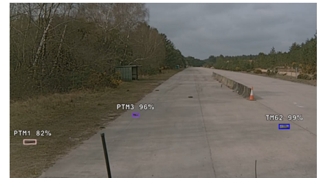
Integration of Threat-Sense by Pearson Engineering is possible – using Artificial Intelligence to identify ordnance
